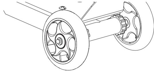
**3** Make sure the locknut, spring washer and small washer are securely tightened against the wheel.
