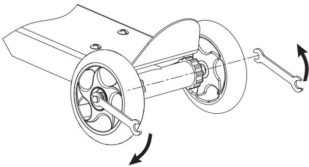
**2** Insert the small washer (3-3), spring washer (3-2) and locknut (3-1) onto the axle bolt and tighten securely using a 10mm wrench.
