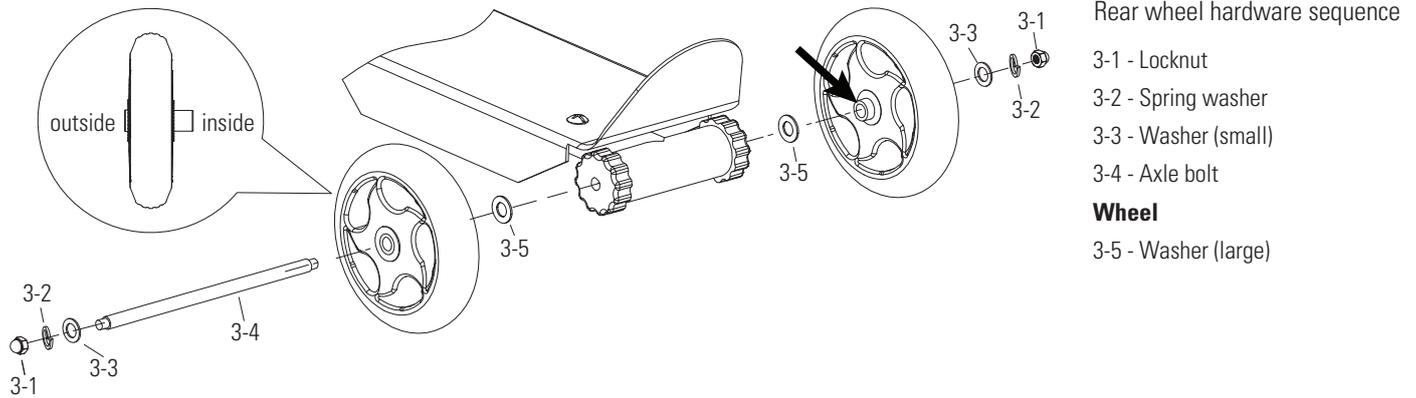
**1** Remove the locknut, spring washer and washers (x3) **from one side** of the axle bolt. Insert the axle bolt through the rear wheel making sure the long spacer on the wheel (refer to arrow above) is facing towards the frame. Insert the large washer (3-5) onto the axle bolt and slide the axle bolt through the frame. Slide the other large washer and wheel (with the long spacer facing inwards towards the frame) onto the axle bolt.
