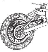
9 Reattach the chain guard using a Phillips screwdriver.
