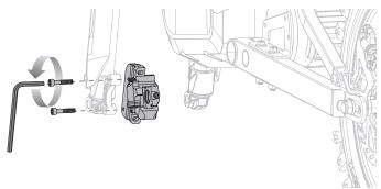
Align the hole in the brake support with the hole in the front fork. Tighten the two (2) bolts using a 5 mm Allen wrench.
