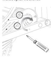
10 Using a Phillips screwdriver, reattach the chain guard.
