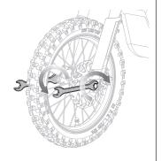
**4** Using a 14 mm and 17 mm wrench, tighten the front wheel.
