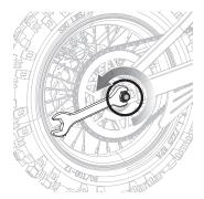
4 Using a 14 mm and a 17 mm wrench, loosen the axle nut then remove the rear wheel assembly.
