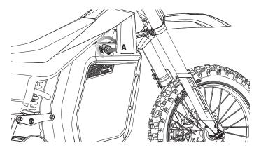
**2** Turn on the power by inserting key **(A)** into the ignition and turning the key clockwise.
