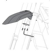
Align fender with the hole in the fork and insert the bolt. Tighten securely using a 5 mm Allen wrench.
