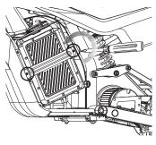
**5** Using a long Phillips screwdriver, remove the two (2) screws from the battery bracket.
