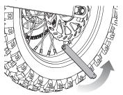
Periodically check that the spokes are tensioned and your wheels are true. Use the included spoke wrench to make adjustments.
