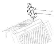
**4** Disconnect the battery connector.
