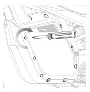
12 Using a long Phillips screwdriver, install the ten (10) screws from left side of the battery box.
