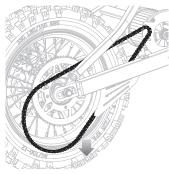
**5** Remove the chain from the wheel sprocket and the motor sprocket.
