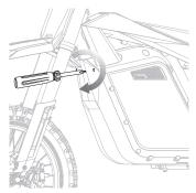
11 Using a long Phillips screwdriver, install the two (2) screws from the front of the battery box.
