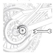
**3** Using a 10 mm wrench, loosen the chain tensioner nut. Loosen the bolt, move the rear wheel forward. Repeat the step on the other side.
