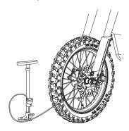
Using a bicycle-style tire pump equipped for a Schrader-type valve, inflate the tires to the correct PSI indicated on the sidewall of the tires.
