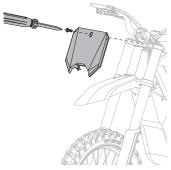
Using a Phillips screwdriver, remove screw from front fork. Align the number plate with the hole in the fork and tighten using a Phillips screwdriver.
