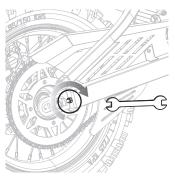
**8** Using a 10 mm wrench, loosen the chain tension nuts (on both sides). Adjust the nut to adjust the chain tightness for both sides. Lock the chain tension nuts. Using a 14 mm and a 17 mm wrench, lock the rear axle.
