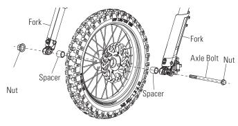
**3** Slide axle through fork, spacer and wheel hub. When axle passes through the other side of the wheel hub, add the other spacer, and slide though the fork. Secure with nut.
