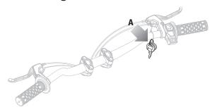
1 Locate key (A) that is on the handlebar.
