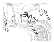
**2** Align the left and right fixing plates with the body bearing holes, put the bolt through the holes one by one. Tighten the bolts and nuts in a clockwise direction using a 10 mm and a 12 mm wrench.
