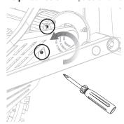
1 Using a Phillips screwdriver, loosen the two (2) screws on the chain guard.
