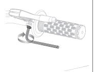
**3** Adjust the brake lever adjuster to the proper place and tighten it with the 5 mm Allen wrench.
