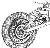
by slipping the chain around the axle. Slide the axle into the slots on the frame. Slide the chain tensioner down and maneuver the chain onto the rear sprocket and motor sprocket.
