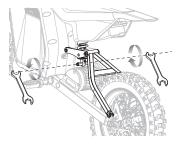
**1** Using a 10 mm and 12 mm wrench, unscrew the screws and nuts as shown.
