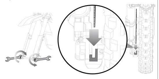
**A WARNING:** Failing to properly adjust and tighten the nuts and bolts that affix the fork can cause you to lose control and fall.
