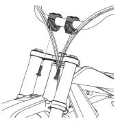
**1** Align the bottom clamp and the top plate on the fork. Lock the bolt from the bottom up, and tighten properly with an 8 mm Allen wrench. Make sure the bottom clamp does not move after tightening.
