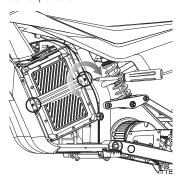
**8** Using a long Phillips screwdriver, install the two (2) screws to the battery bracket.
