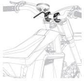
**2** Adjust the handlebars in the clamps as needed and tighten. Make sure the handlebars don't move after tightening.
