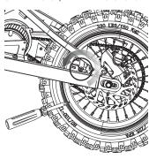
**2** On the other side, using a Phillips screwdriver, remove the screw.
