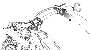
**3** Sit on the electric motor bike seat with both feet on the ground on either side of the seat to balance the unit. Place both hands on the handlebars and apply the throttle **(B)**.
