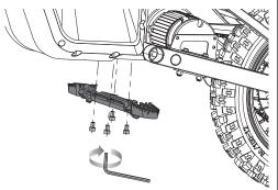
Align the hole in the foot pegs with the hole in the frame and tighten the four (4) bolts using a 6 mm Allen wrench.
