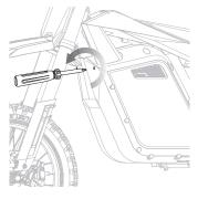
**2** Using a long Phillips screwdriver, remove the two (2) screws from the front of the battery box.
