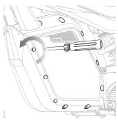
1 Using a long Phillips screwdriver, remove the ten (10) screws from left side of the battery box.
