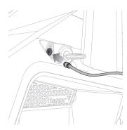
**2 Note:** Make sure power button is in the **OFF** position. Plug the charger into the charger port. The light on the charger should turn red during charging. The light will turn green again when charging is complete.
