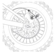
**1** To adjust brake cable play, thread the brake lever adjuster in or out 1/4 to 1/2 turn until the desired brake adjustment is attained. Most adjustments are complete at this step. If brake still needs further adjustment, proceed to step 2.
