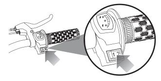
Pressing the "1" on the speed switch sets the HIGH setting. Pressing the "2" on the speed switch sets the LOW setting.
