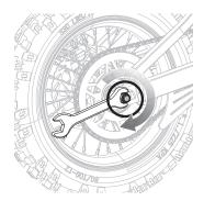
**7** Using a 14 mm and a 17 mm wrench, tighten the axle nut.
