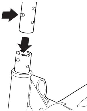
**4** Insert the T-bar into the front fork assembly using your thumb to depress the button on the T-Bar until it "locks" into place.
