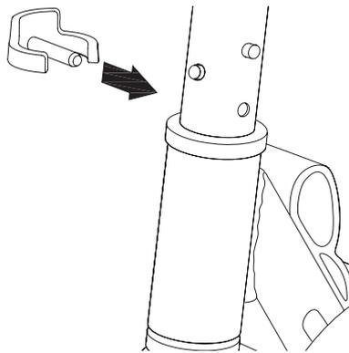
**5** Insert the "E" shaped fixed pin into the open hole on the front fork assembly to secure T-bar.
