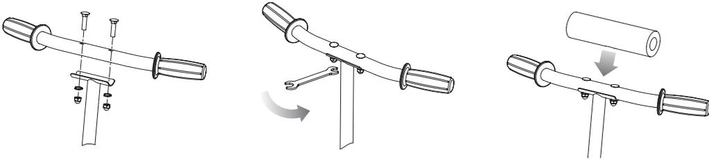
**1** Align the holes on the handlebar and the T-bar. Insert handlebar bolts into the top of the handlebar and through the T-bar. Install the washers and nuts onto the bottom of the handlebar bolts. Tighten securely into place using a 10 mm wrench.
