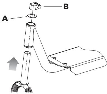
**1** Remove the black protective cover from the top of the fork. Using a 13 mm wrench, loosen collar clamp bolt and slide collar clamp (B) up the fork and remove. Remove washer (A) from fork. Insert the front fork into the steering tube. Slide washer (A) back onto the front fork. Slide collar clamp (B) back down onto the fork until it is sitting directly on top of washer (A).
