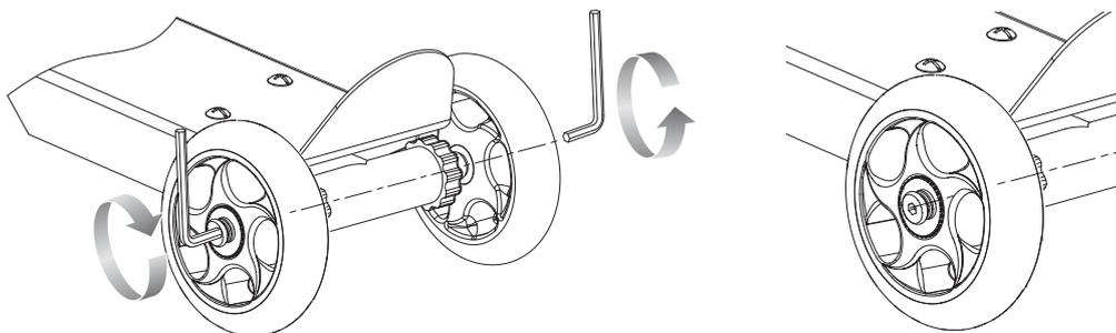
**2** Tighten securely using two (2) 5 mm Allen wrenches.
