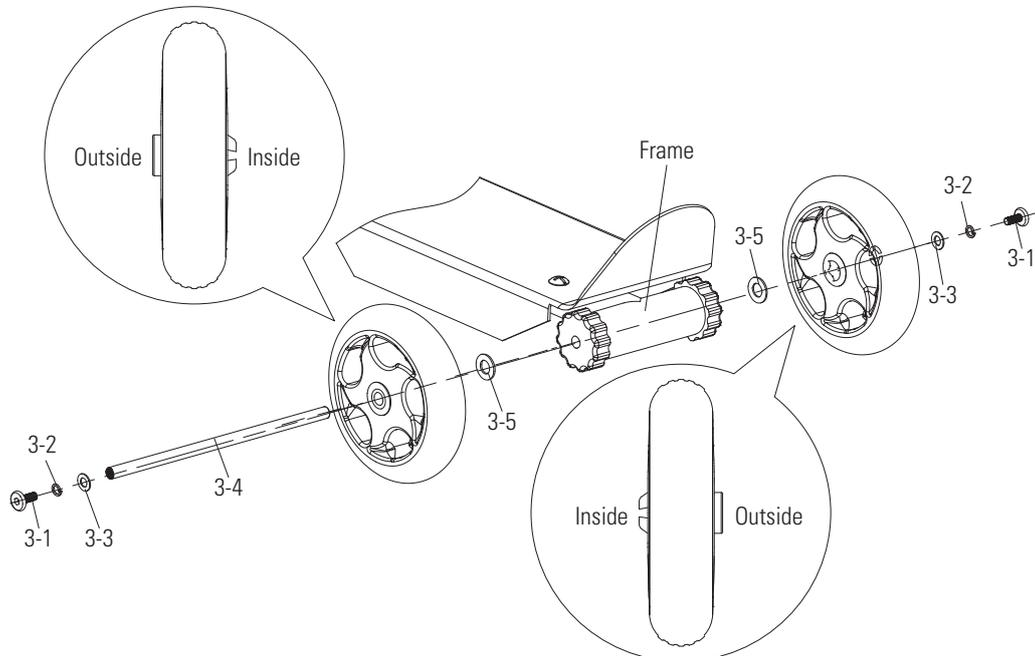
**1** Remove the locking screw (3-1), spring washer (3-2), small washer (3-3) and large washer (3-5) **from one side** of the axle bolt. Insert the axle bolt through the rear wheel. Insert the large washer (3-5) onto the axle bolt between the frame and rear wheel and slide the axle bolt through the frame. Slide the other large washer and wheel onto the axle bolt.
