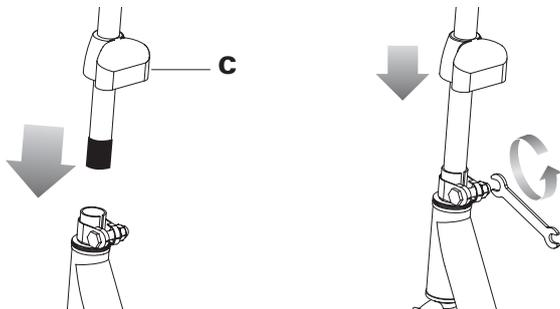
**1** Slide collar clamp cover (C) up to the middle of the T-bar. Insert the T-bar all the way down into the front fork.
