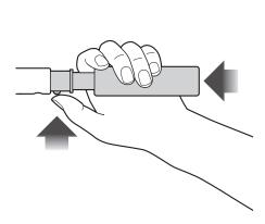
**3** Insert and secure the left and right handlebars by pressing the spring-loaded buttons and inserting them into the T-bar.
