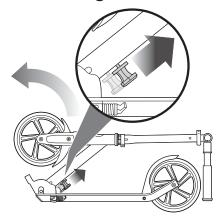
**1** To release the folding mechanism, place the scooter on the ground. Slide the Anti-Rattle knob up to raise T-bar. Turn knob completely counterclockwise and continue raising T-bar until it is locked in the upright position.
