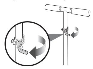
**1** To adjust the height of the handlebars, open the quick-release lever and slide the T-bar to the desired position and resecure the quick-release lever to lock into place.
