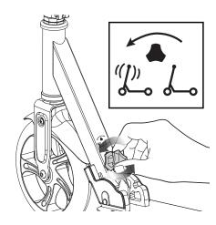
1 To fold scooter you must first deactivate the Anti-Rattle feature. Turn the knob counterclockwise to loosen.
