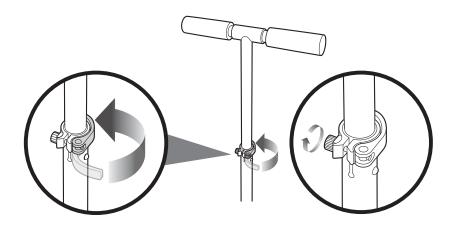
**2** The tension of the quick-release lever can be adjusted by manually tightening or loosening the Allen bolt. Be careful not to over-tighten. You should always be able to open and close the quick-release lever by hand and the T-bar should slide freely when the quick-release lever is open.
