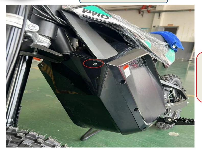
Use a Philips screwdriver to remove the screw from the battery front cover.
