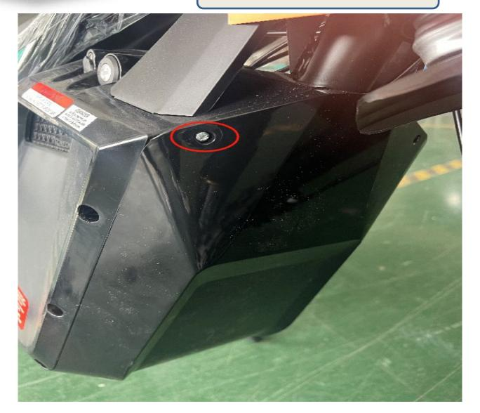
Use a Philips screwdriver to remove the screw from the battery front cover.
