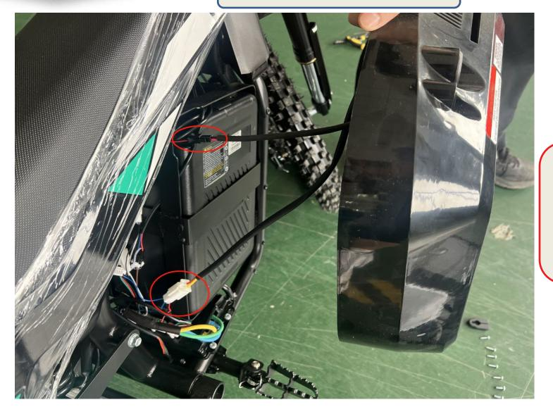
Take the right battery cover down after unplugging the charge port plug and power switch plug.
