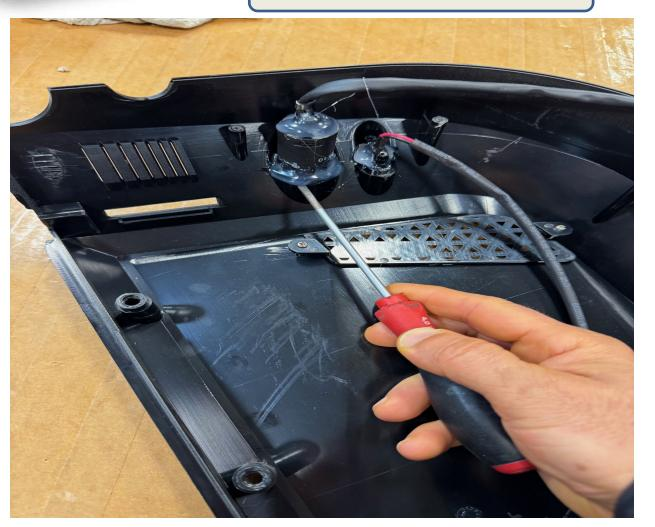
Using a Flat screwdriver remove the glue at the back of the power switch and push the switch out from the cover.
