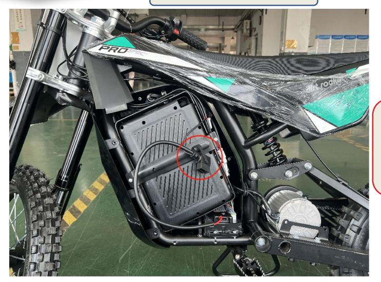
Disconnect the battery connector.
