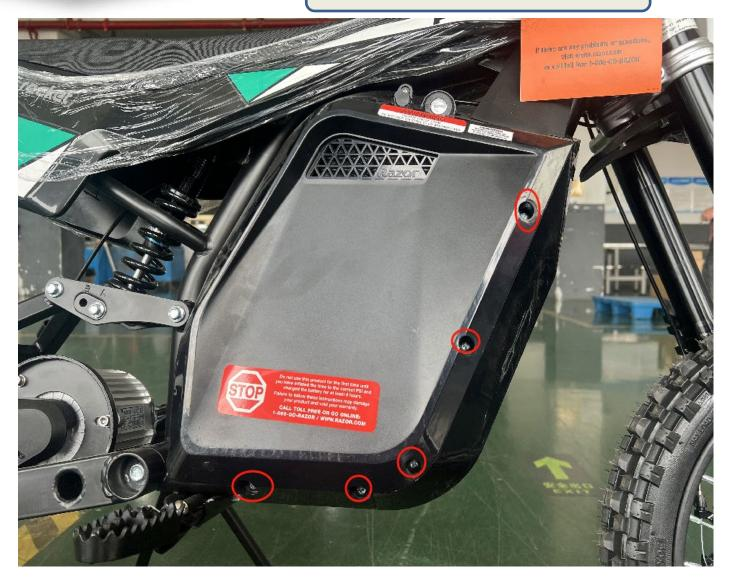
Use a Philips screwdriver to remove 5pcs screws from the right battery cover.
