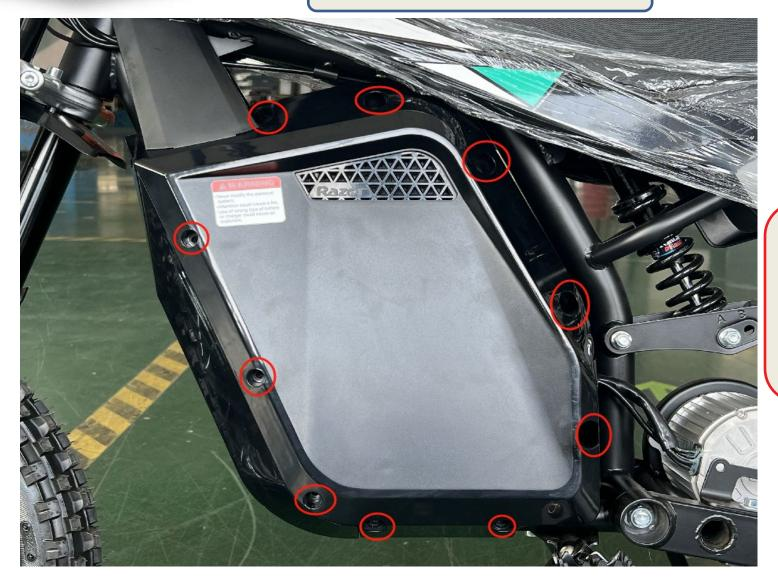
Use a Philips screwdriver to remove 10pcs screws from the left battery cover.
