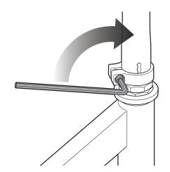
**AWARNING:** Failure to properly install and tighten the collar clamp may cause the rider to lose control and fall. If you are having difficulty understanding these instructions, please contact Razor Customer Service for assistance.
