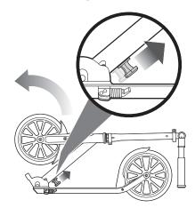
**1** To release the folding mechanism, place the scooter on the ground. Slide the Anti-Rattle knob up to raise T-bar. Turn knob completely counterclockwise and continue raising T-bar until it is locked in the upright position.
