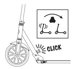
**2** Turn knob clockwise to tighten and engage the Anti-Rattle mechanism.
