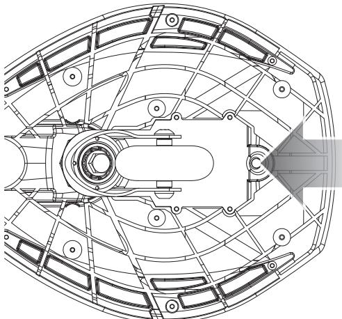
**4** Insert the new AA batteries and replace the cover and four (4) screws using a Phillips screwdriver.
