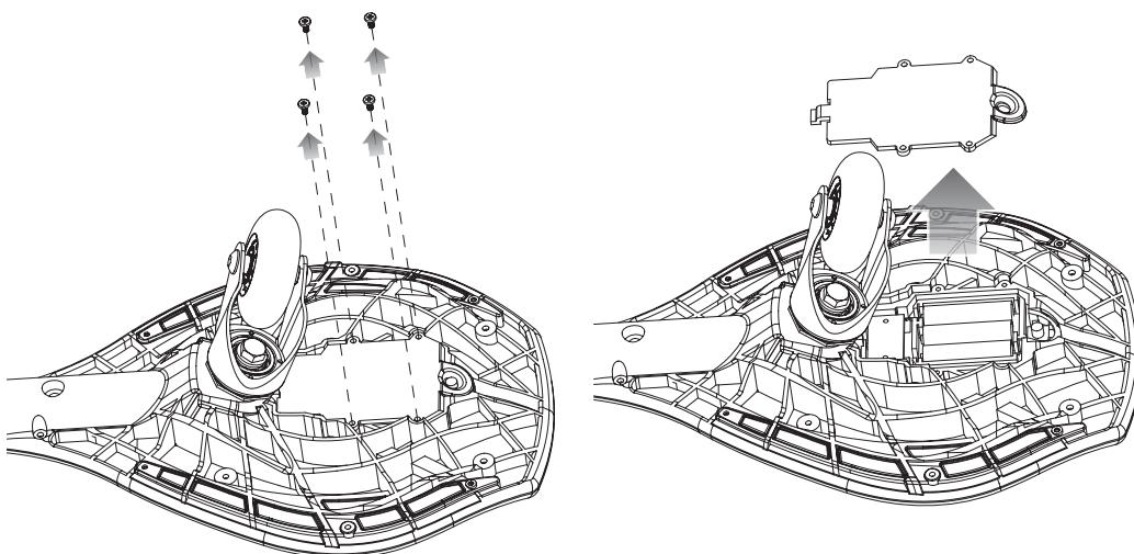
**1** Using a Phillips screwdriver, remove the four (4) screws from the battery cover.
