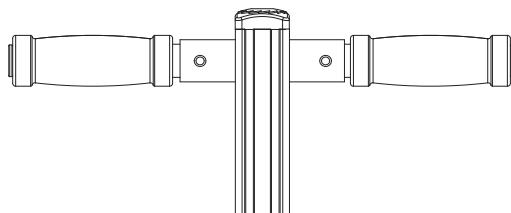
**2** Make certain **BOTH** handlebars are properly locked onto the main shaft.
