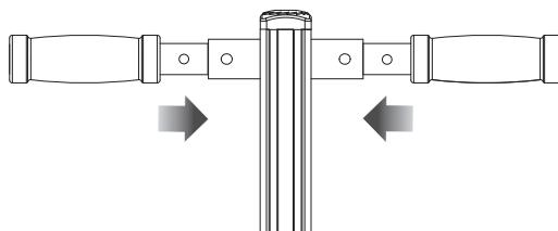
**1** Insert and secure the left and right handlebars by pressing the spring-loaded buttons and inserting them into the main shaft.
